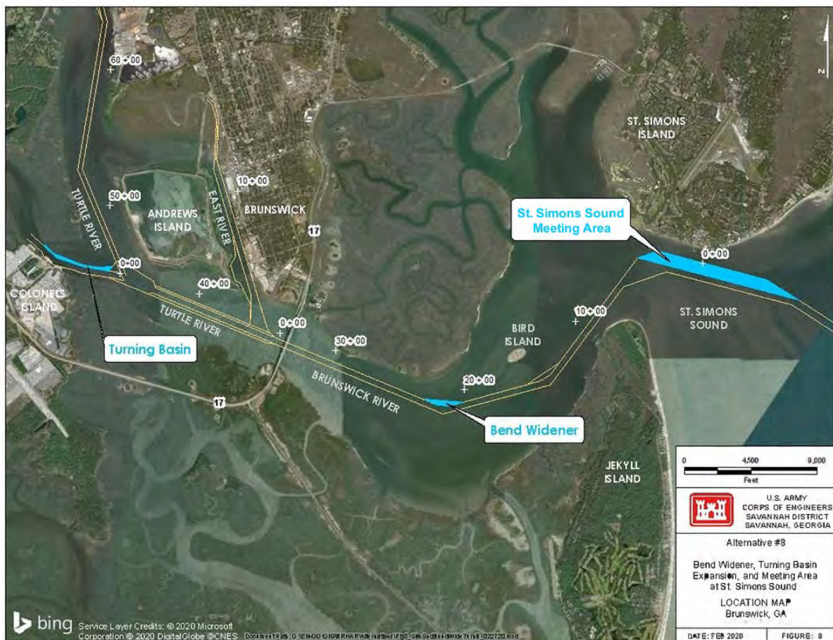
Figure 1. BHMP locations of widening areas. The bend widener consists of mostly sandy material and is suitable for beneficial use. The turning basin consists of mostly fines and is not suitable for beneficial use. The St. Simons Meeting Area does not require removal of material.
